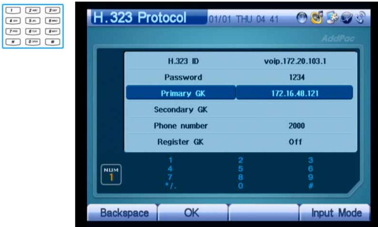
(Figure 3-154) Entering IP Address of Primary Gatekeeper
