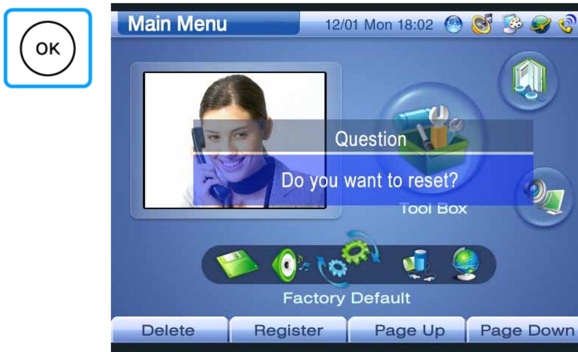
(Figure 3-66) Pressing the “OK” Button for Three Seconds After Selecting the Factory Default Menu
