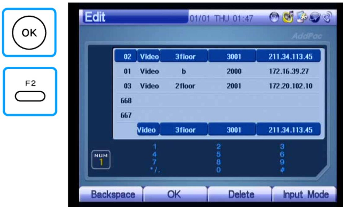
(Figure 3-31) Completing Input by Pressing the “OK” Button of Keypad
