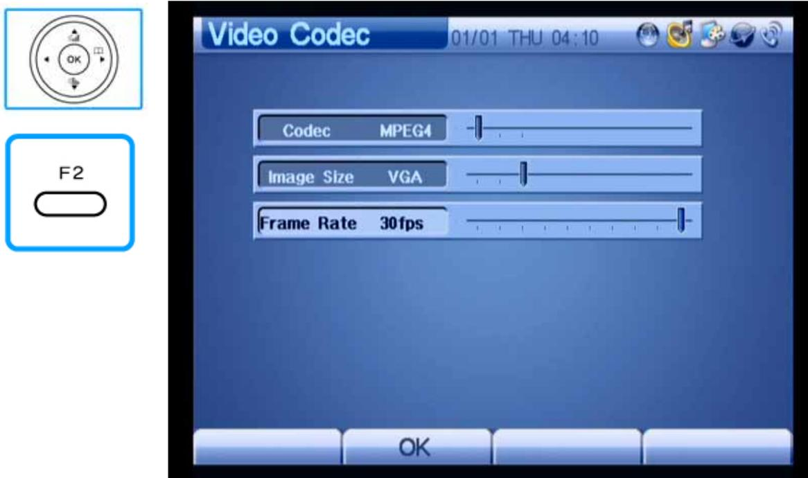
(Figure 3-105) Setting Frame Rate to 30 fps
