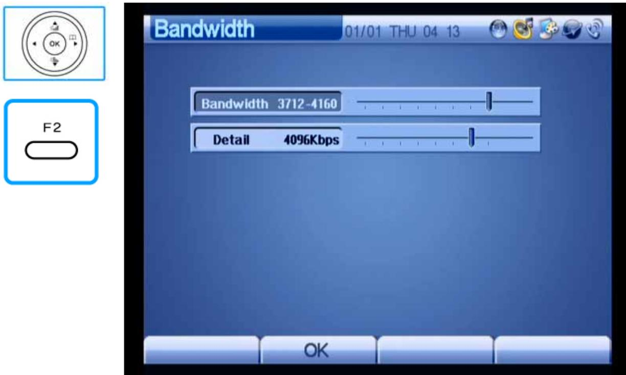
(Figure 3-112) Setting the Bandwidth in Detail to 4096 Kbps
