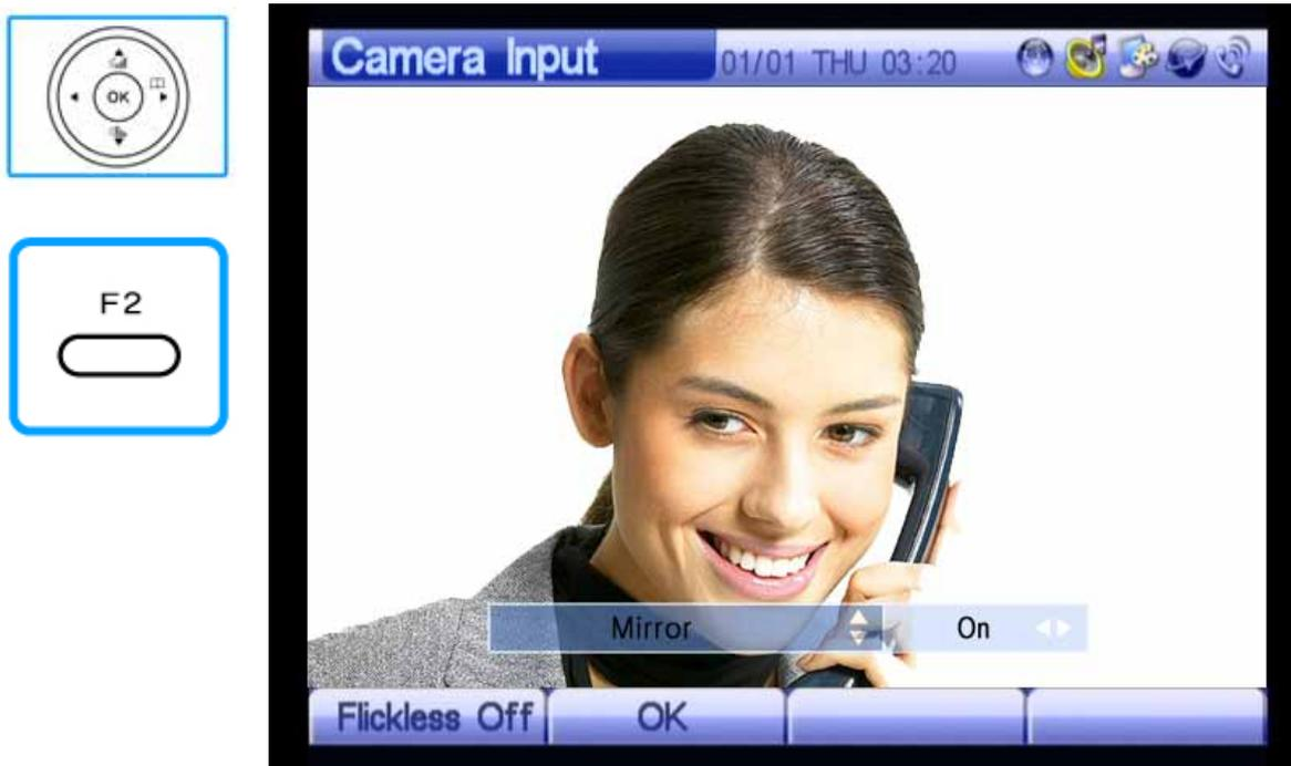
(Figure 3-87) Inverting Camera Input Left or Right
