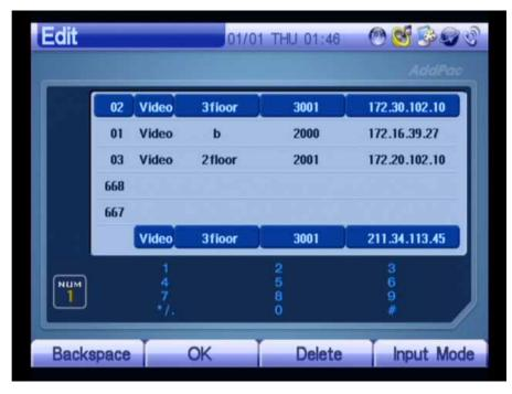
(Figure 3-30) Changing the IP Address to "211.34.113.45"
