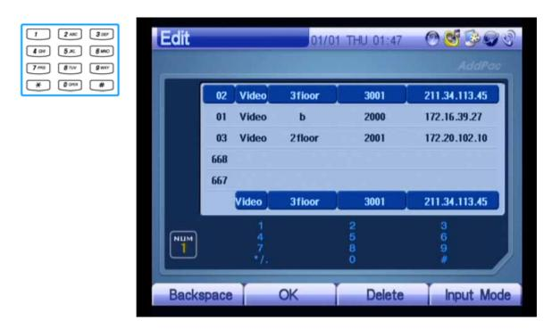
(Figure 3-37) Selecting Audio/Video Session Using Number Keys of Keypad
