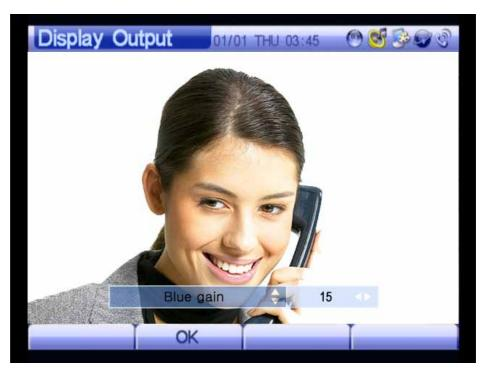
(Figure 3-93) Adjusting Blue Gain
