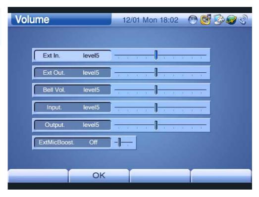
(Figure 3-74) Adjusting Audio Input Volume to 5
