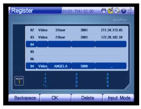
(Figure 3-43) Moving to the IP Address by Pressing the OK Button of Keypad
