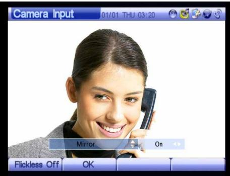
(Figure 3-87) Inverting Camera Input Left or Right
