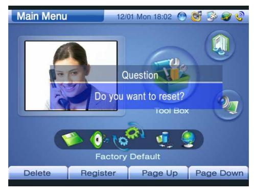
(Figure 3-66) Pressing the "OK" Button for Three Seconds After Selecting the Factory Default Menu
