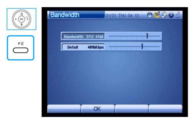
(Figure 3-112) Setting the Bandwidth in Detail to 4096 Kbps
