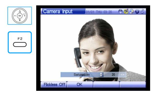
(Figure 3-86) Adjusting Saturation by Using the F2 Button of the Keypad
