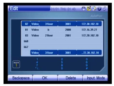
(Figure 3-29) Moving to IP Address By Pressing the OK Button of Keypad
