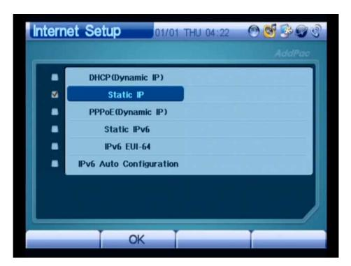
(Figure 3-129) Selecting Static IP
