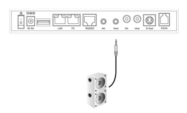
(Figure 3-5) Connection of Audio Output Interface to AP-VP150
