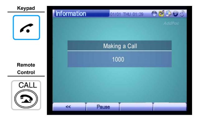
(Figure 4-5) Making a Call Using the Call Button
