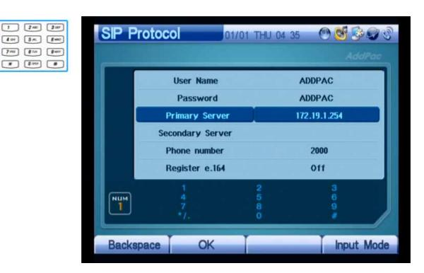
(Figure 3-149) Entering IP Address of Primary Server
