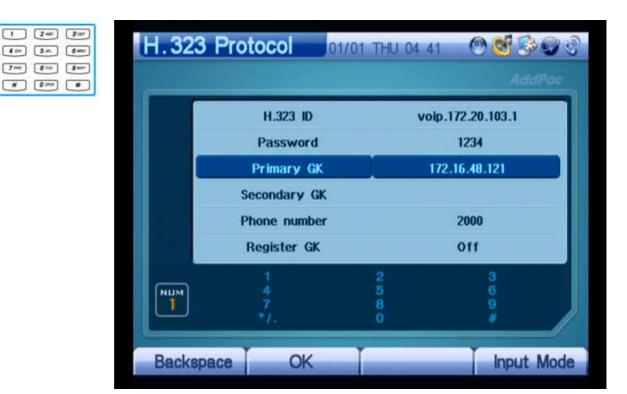
(Figure 3-154) Entering IP Address of Primary Gatekeeper
