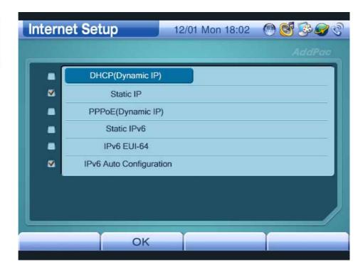
(Figure 3-126) Pressing the "OK" Button After Selecting DHCP
