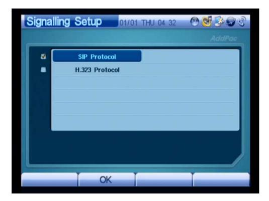
(Figure 3-145\_2) Signalling Setup Screen
