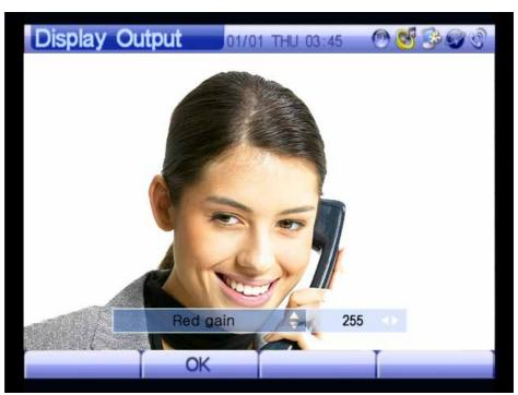
(Figure 3-94) Adjusting Red Gain
