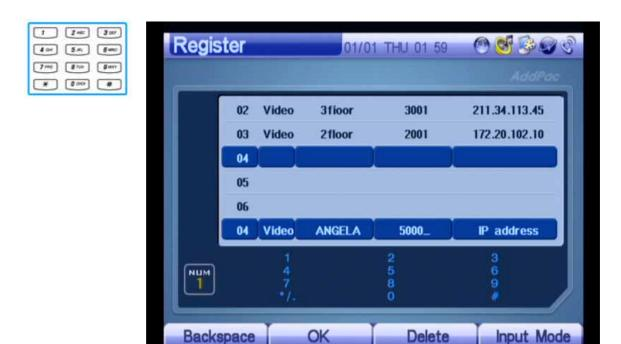
(Figure 3-44) Entering "213.23.112.32" as IP Address
