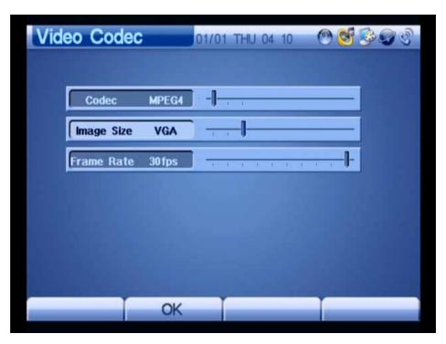
(Figure 3-104) Setting Image Size to VGA
