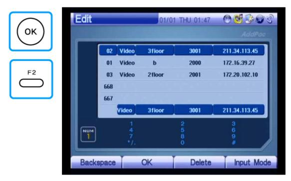
(Figure 3-31) Completing Input by Pressing the "OK" Button of Keypad
